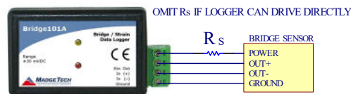
Figure 10, The packaged bridge configuration for 4-wire Bridge products
